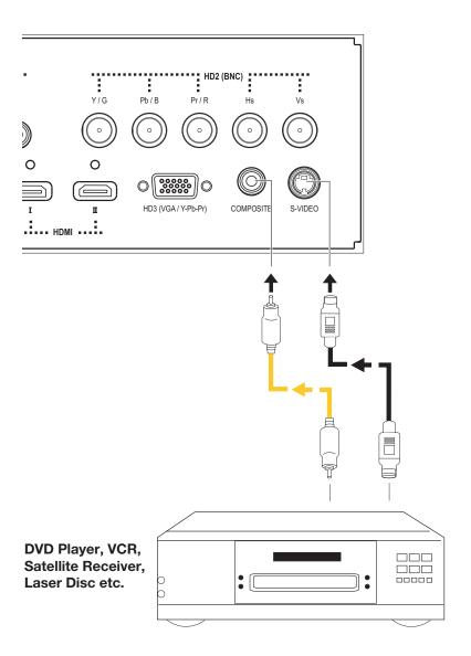
Figure 3-15. S-Video and Composite Video Connections
